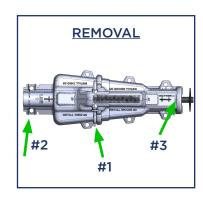
"#2" indicated loop. Pull Half 2 off completely. Next, pull upwards on Half 1 at "#3" green arrow indicated loop to release Half 1 from Guard Clamp. Lastly, unscrew and remove Guard Clamp by using a 15/16" wrench or socket.
